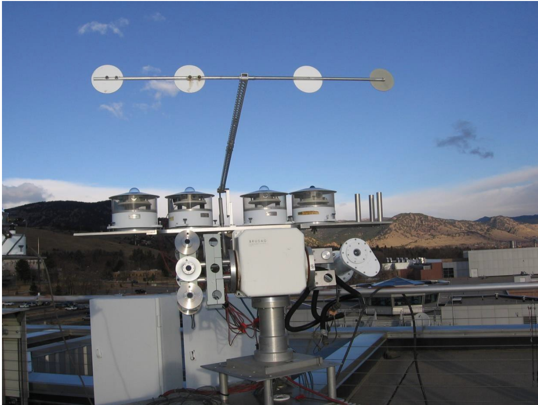
Diffuse and direct solar radiation instrument calibrations at the NOAA GMD Boulder, Colorado rooftop facility.
