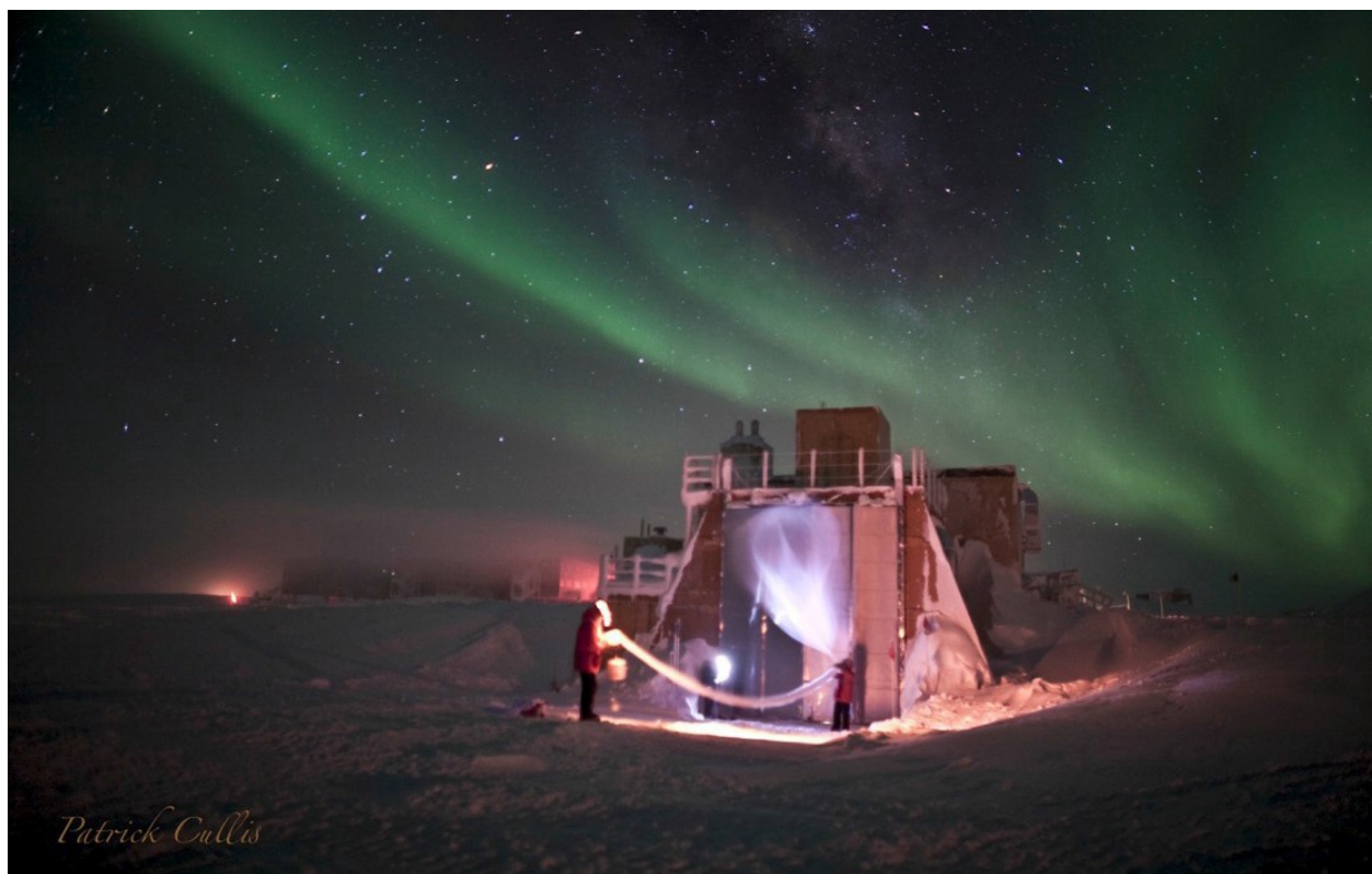
GMD South Pole staff releasing a large plastic balloon carrying an ozonesonde to measure stratospheric ozone concentrations. Temperature -80^{\circ}\text{F} ( -62^{\circ}\text{C} ).
